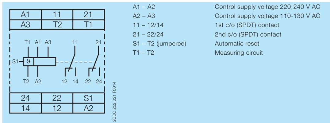
Connection diagram CM-MSS.33
