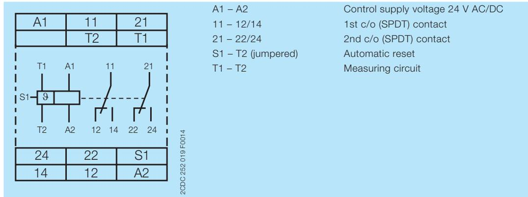
Connection diagram CM-MSS.32
